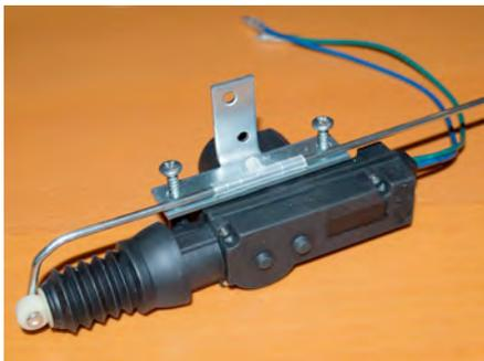
Then I cut the rod to an appropriate length, affixed a large cable tie to its end to work as a pulley on the lock release and joined all pieces with two small cable ties to the bracket, using a remainder of the large cable tie as spacer.
