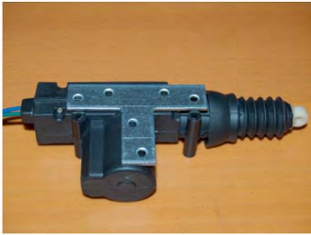
Here is a close look of the bracket from our local DIY store, the holes almost perfectly matching the mounting points of the solenoid. Only very little work had to be done with the file after bending it:
