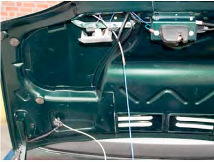
It is now time to connect the solenoid to the long blue cable that has to be fiddled through to the cigar lighter. A wiring aid for electric installations can be quite handy here. I used this to pull the wire through the boot lid from the boot lamp as well as from the engine compartment to the rear shelf.
