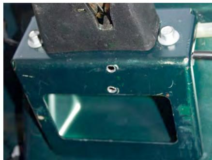
My first idea was to cut threads into the holes and fix the bracket with two of the three M4 clamp screws from the kit. But I didn't have a 3.2 mm drill handy in the first place and even more it seemed a bit tricky, as there will be quite some force applied here.
