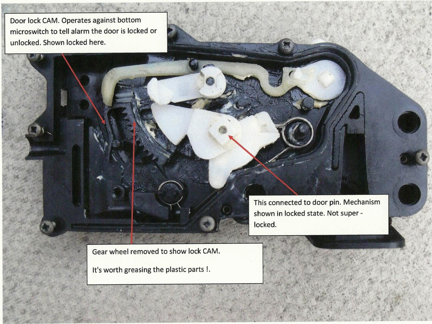
This connected to door pin. Mechanism shown in locked state. Not super - locked.
