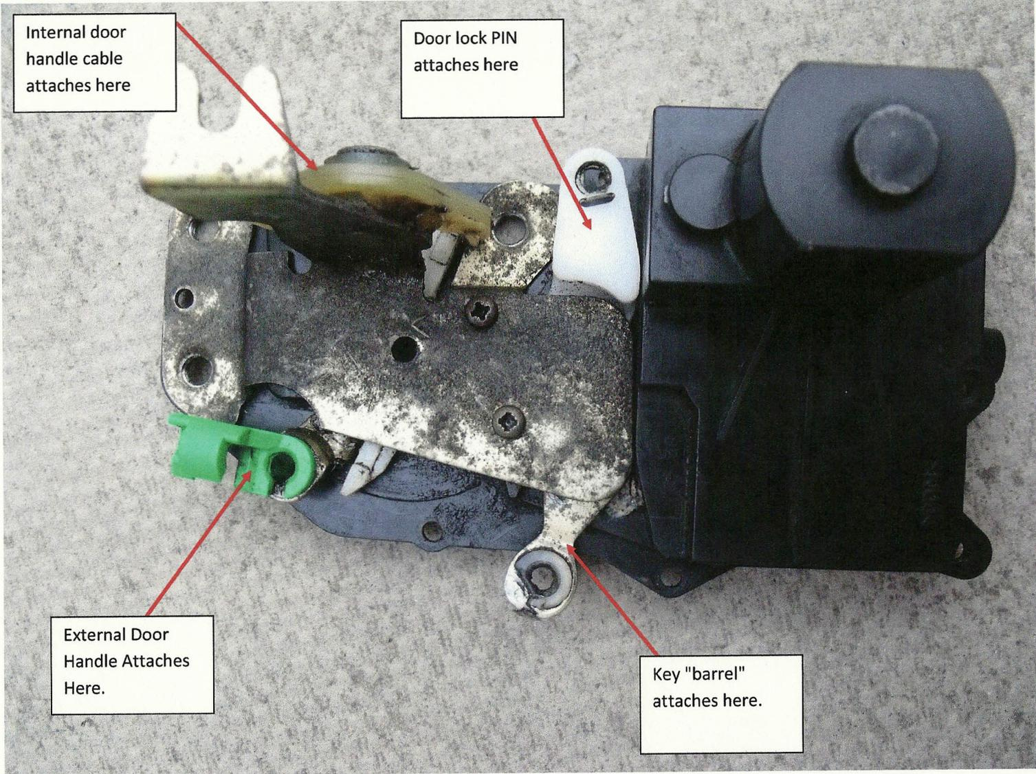
Internal door handle cable attaches here
